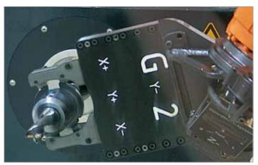
Cleaning unit for machine taper cleans the tool shaft; This results in higher precision and concentricity of the tools. Available for all standard tool holders.
