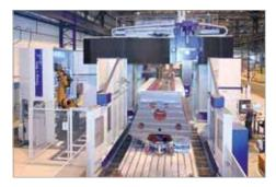
Tool capacity 280 pieces Workpiece loading stations 16 pieces max. tool length 1000 mm max. tool diameter 400 mm max. tool diameter (bridge-type) 800 mm max. tool weight 100 kg
