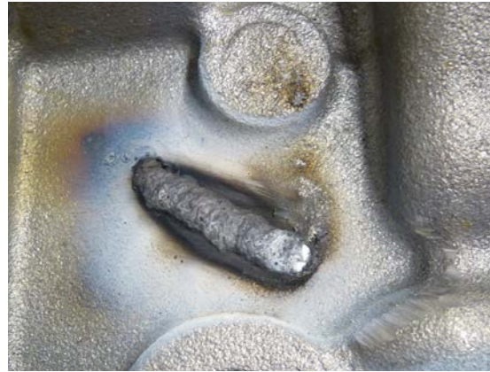
Short stringer bead before slag is removed
