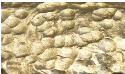
Hammered out weld metal
