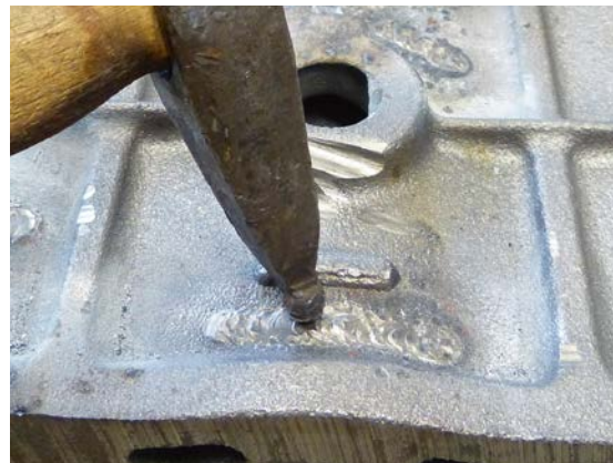
Short stringer bead after slag is removed
