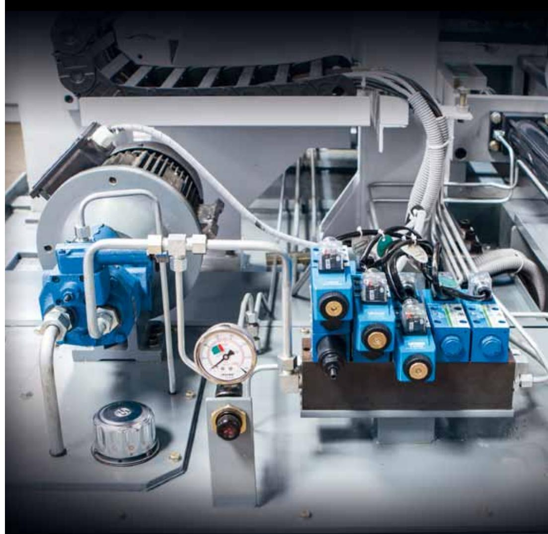
**CENTRALINA IDRAULICA DI ULTIMA GENERAZIONE, AD ELEVATA EFFICIENZA E BASSO CONSUMO ENERGETICO.**
